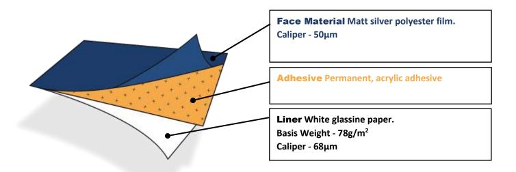
**General** #863 is a metalized polyester film with a matt surface. The film is treated with a special top coating for printing. The feature of this product is the film delaminates and releases an adhesive layer with the writing 'VOID'. The removed film is completely free from adhesive once removed. The writing is only partially visible until the label is removed.
