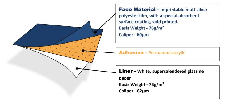
**General** #789a is an imprintable matt silver polyester film, with a special absorbent surface coating, void printed. The adhesive is perfectly suitable for uses that need a good resistance to UV, fats or solvents. Good general adhesion performance on a wide range of substrates.
