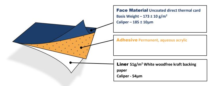
**General** #826 / #1167r is an uncoated direct thermal card card with standard sensitivity giving up to 7 years image durability. It has a permanent adhesive and a white, woodfree kraft backing paper
