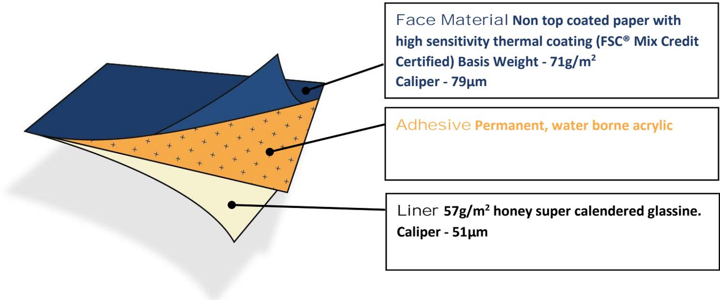
**General #704r** is a paper with a high sensitivity thermal coating produced totally without BPA-based chemistry. The pulp for this paper comes from FSC certified forest management and other controlled sources. Limited resistance to thermal image scratching or smudging.
