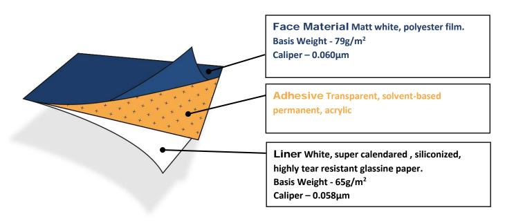
**General** #585 is a matt white polyester film. The surface is covered with a matt topcoat designed for thermal transfer printing. The adhesive is a transparent, solvent-based permanent, acrylic adhesive. It is distinguished by very high ageing stability and it features very high resistance against chemicals and heat. The liner is a white, supercalendered, siliconized, highly tear-resistant glassine paper with very good die-cutting properties. This liner is not recommended for fanfolding.
