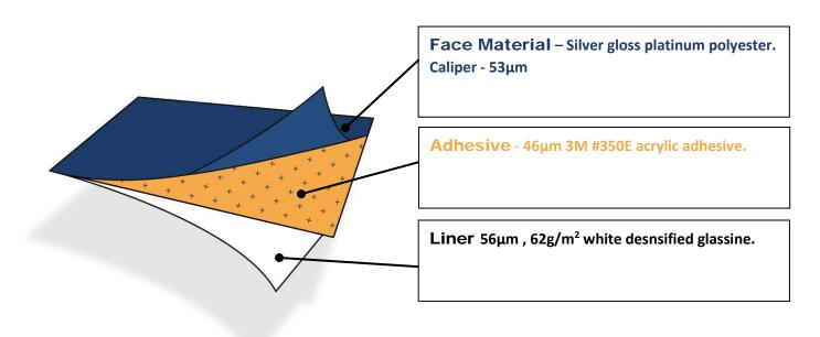
**General** #584 is a silver gloss platinum polyester facestock with a topcoat for thermal transfer printing, resin ribbons are recommended for optimum durability. #350E adhesive is 3M's most universal labelstock adhesive offering excellent adhesion, even on low surface energy substrates combined with excellent temperature and chemical resistance.
