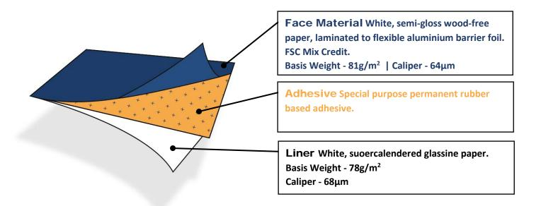
**General** #240a is a white coated, wood-free printing paper with semi-gloss appearance, laminated to a flexible aluminium barrier foil.
