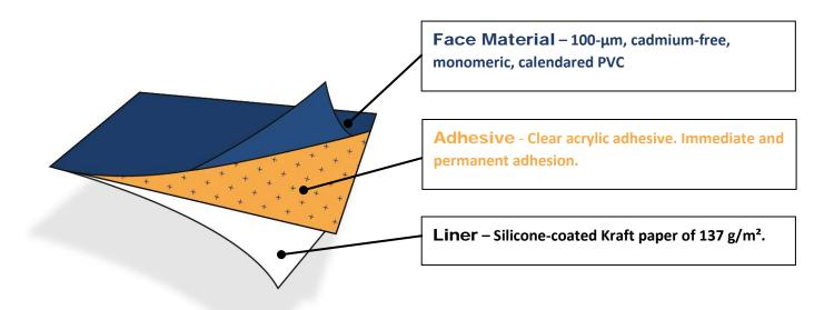
**General** #970 is a  $100-\mu m$  cadmium-free, monomeric, calendered PVC which is coated with a clear pressure-sensitive, acrylic adhesive. The adhesive is resistant to most chemical agents (alcohol, diluted acids, oils).
