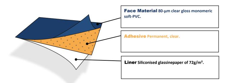
General #833c is an 80-µm gloss clear monomeric soft-PVC with a clear permanent adhesive
