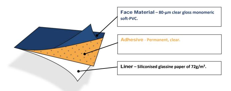
General #833c is an 80-µm gloss clear monomeric soft-PVC with a clear permanent adhesive
