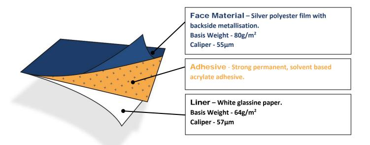
**General** #219 is a silver polyester film with backside metallisation. The surface is covered with an absorbing, matt topcoat for very good ink anchorage. It is distinguished by very high ageing stability and features excellent resistance against chemicals, heat and UV light. It has a high peel adhesion on high and medium surface energy substrates.
