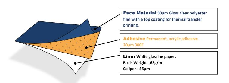
**General** #184 is a gloss clear polyester film with a top coating for thermal transfer printing. Resin ribbons are recommended for optimin durability. The facestock provide durability in harsh environments.
