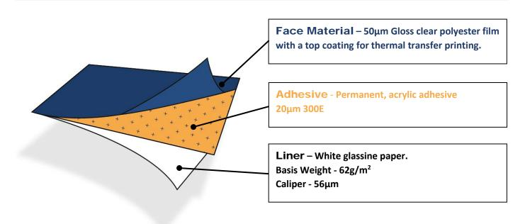
**General** #184 is a gloss clear polyester film with a top coating for thermal transfer printing. Resin ribbons are recommended for optimin durability. The facestock provide durability in harsh environments.
