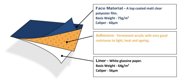
**General** #168 is a matt clear computer imprintable polyester film with a top coating for better printability. The matt surface offers an excellent quality of the imprint by screen, letterpress and flexo printing. Also suitable for thermal transfer and laser printers after production.
