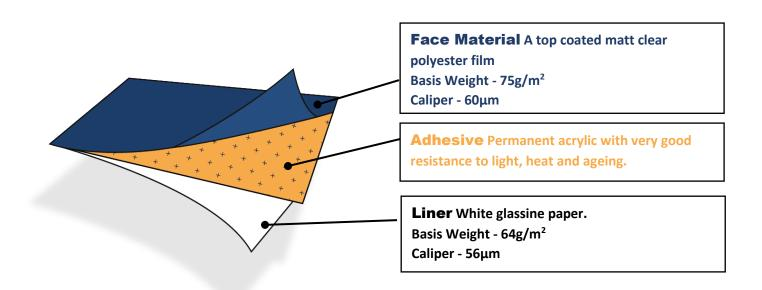
**General** #168 is a matt clear computer imprintable polyester film with a top coating for better printability. The matt surface offers an excellent quality of the imprint by screen, letterpress and flexo printing. Also suitable for thermal transfer and laser printers after production.
