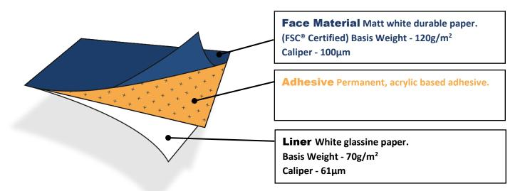
**General** #1312 is a durable matt white material with a paper-feel to it. It contains 80% calcium carbonate bonded with 20% HDPE.
