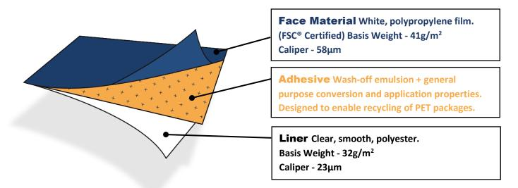
**General** #1311 is a white, polypropylene film. The film is orientated biaxially and has a good print-receptive finish.
