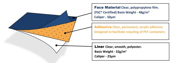
**General** #1310 is a clear, polypropylene film. The film is orientated biaxially and has a good printreceptive finish.
