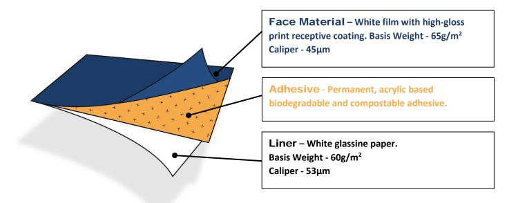
**General** #1307 is a white, high-gloss film with a print receptive coating. It is produced from wood pulp sourced from managed plantations. Good initial tack and adhesion on wide variety of substrates.
