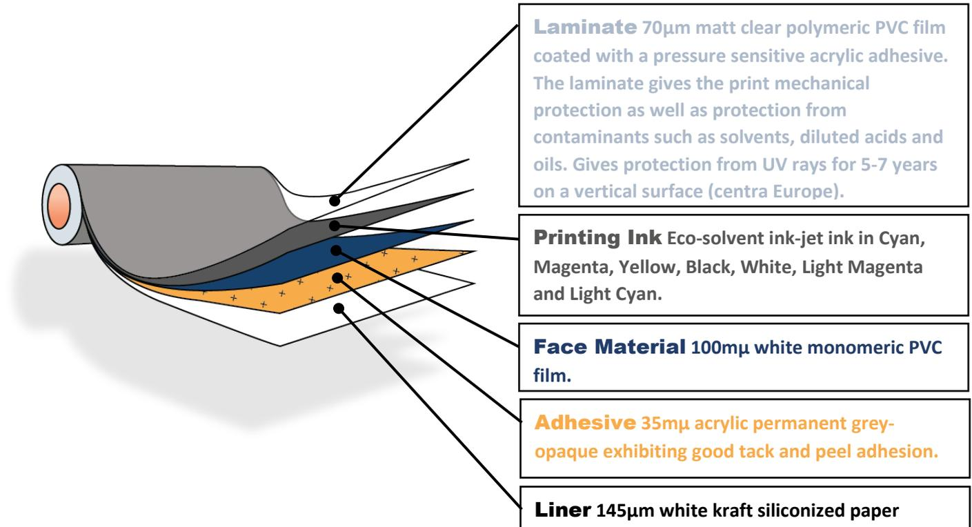
**General** All size labels, decals and rolls up to a maximum of 1,250mm wide. 210µ total construction thickness, durable soft monomeric vinyl coated with high-tack permanent grey-opaque self-adhesive. Printed with solvent ink-jet CMYKLcLmW which can include barcode and human readable variable fields - either sequential or from customer database - and laminated with clear vinyl perm.
