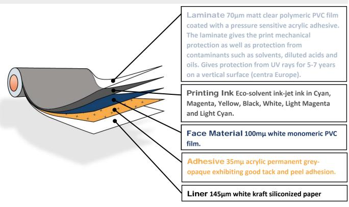
**General** All size labels, decals and rolls up to a maximum of 1,250mm wide. 210mµ total construction thickness, durable soft monomeric vinyl coated with high-tack permanent grey-opaque self-adhesive. Printed with solvent ink-jet CMYKLcLmW which can include barcode and human readable variable fields either sequential or from customer database - and laminated with clear vinyl perm.
