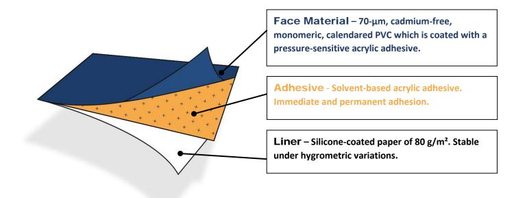
**General** #833 is a protective film enabling you to modify the substrates appearance by providing it with a matt surface finish. It is UV proof and resistant against mechanical wear. We strongly advise against #833 when using **v880 and v890.**
