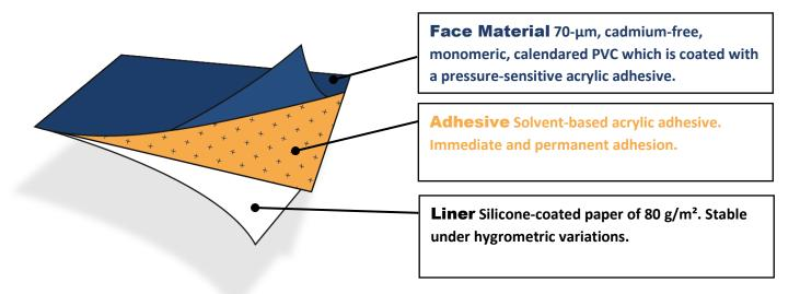
**General** #833 is a protective film enabling you to modify the substrates appearance by providing it with a matt surface finish. It is UV proof and resistant against mechanical wear. We strongly advise against #833 when using **v880 and v890.**
