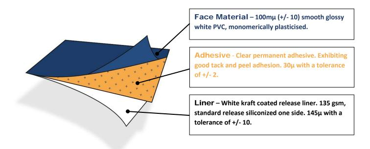
**General** #374b is a smooth glossy white PVC laminated with an extra-permanent, low shrinkage, clear acrylic adhesive. The PVC is suitable for printing by eco-solvent and solvent based inks and has a minimum outdoor life of 2 years.
